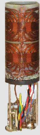
Vertical Bore MRI Probe with 3 axis gradients and a RF *Litz* or *Litzcage* coil
