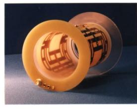
The *Litz* (woven) coil utilizes etched foil patterns with insulated crossovers to obtain *rf* flux transparency and improved S/N. Special symmetries permit an ideal current distribution that is largely independent of tuning, matching, and balancing adjustments. Homogeneity is excellent and tuning is simple.
