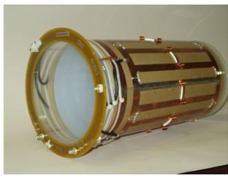
Doty *Litzcage* coils combine the Circular-Polarization (CP) of a *rf* birdcage coil and the insulated crossovers of the Doty *rf Litz* coil to produce a superior quadrature coil with easy tuning.
