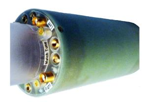
Mouse Coil, <sup>1</sup>H at 646 MHz for a 15.2 T Horizontal Bore Imager with a 6 cm Bore, 36 mm ID x 50 mm Length (59 mm OD)
