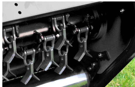
Y-shaped mounting of knives on shackles
