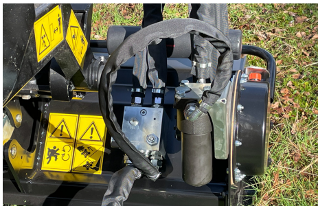
Safety hydraulic block with Cartridge filtration
