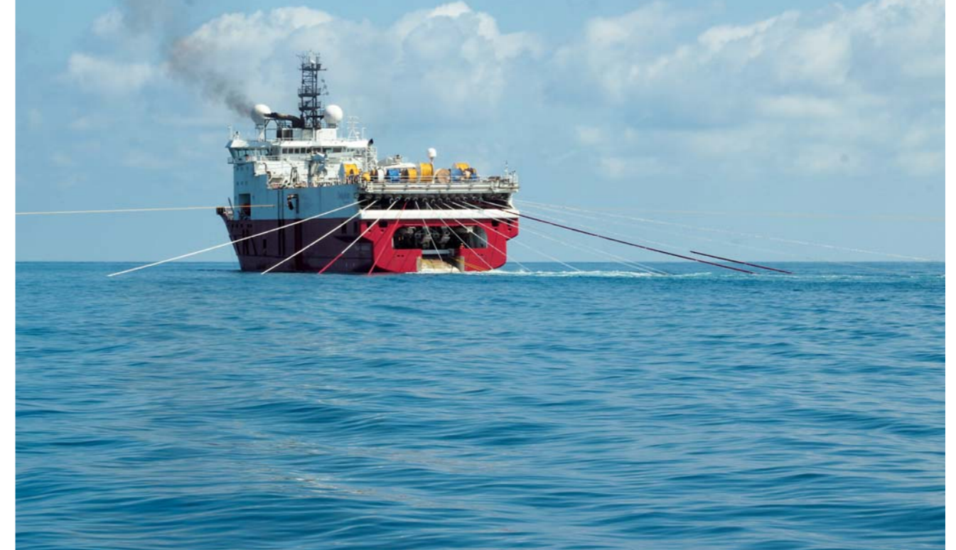
Offshore 3D seismic surveys in the Black Sea
