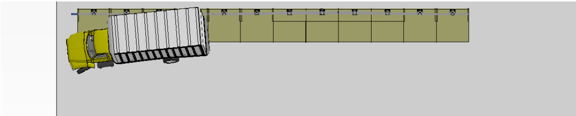
Figure M-1. [Continued] Sequential views from analysis of MASH Test 4-12 for sidewalk-mounted S3-TL4 from an overhead viewpoint (Case 1).
