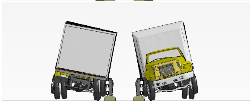
Figure J-2. Sequential views from analysis of MASH Test 4-12 for curb-mounted S3-TL4 from upstream and downstream viewpoints (Case 1).
