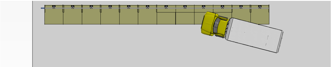
Figure M-1. Sequential views from analysis of MASH Test 4-12 for sidewalk-mounted S3-TL4 from an overhead viewpoint (Case 1).
