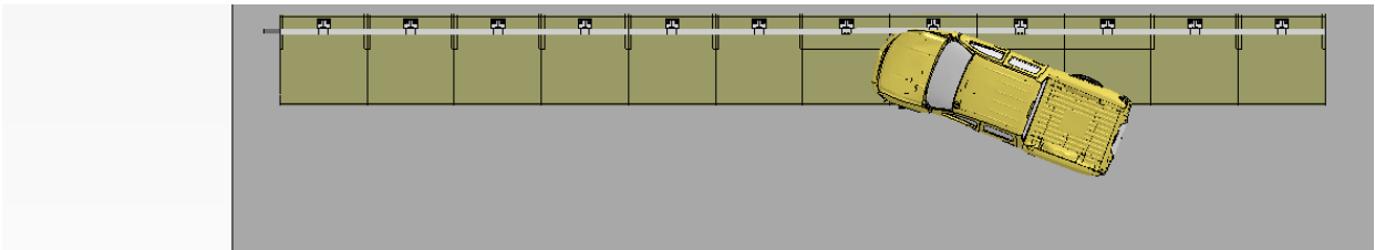
Figure I-1. Sequential views from analysis of MASH Test 4-11 for sidewalk-mounted S3-TL4 from an overhead viewpoint.
