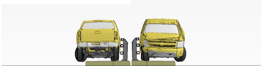
Figure I-2. Sequential views from analysis of MASH Test 4-11 for sidewalk-mounted S3-TL4 from upstream and downstream viewpoints.
