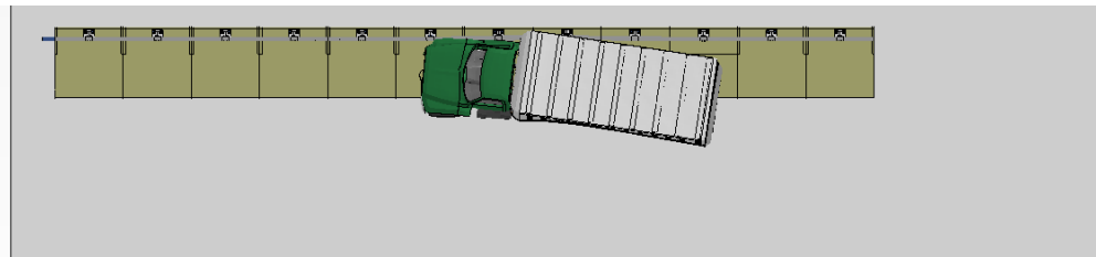
Figure N-1. [Continued] Sequential views from analysis of MASH Test 4-12 for sidewalk-mounted S3-TL4 from an overhead viewpoint (Case 1).
