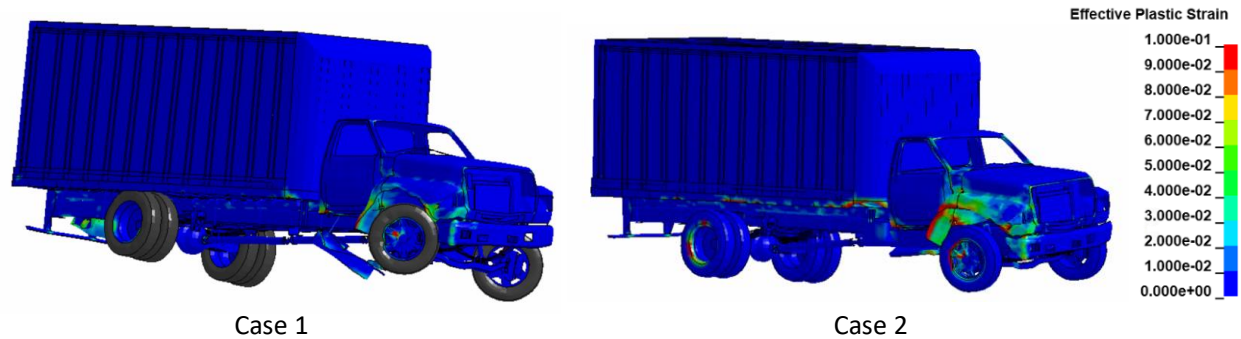
Figure 113. Damages to vehicle in Test 4-12 analysis of curb-mounted bridge rail for Cases 1 and 2.
