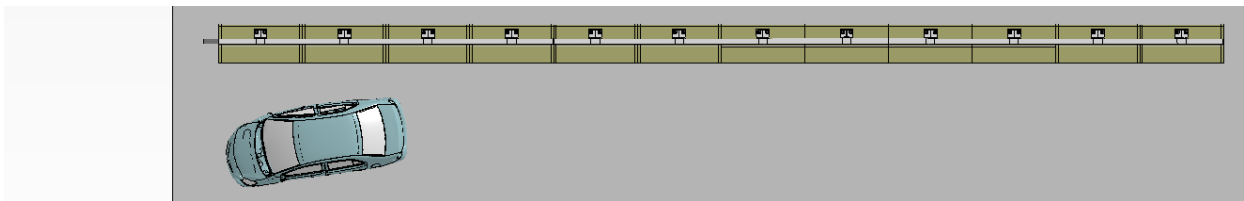
Figure F-1. [Continued] Sequential views from analysis of MASH Test 4-10 for curb-mounted S3-TL4 from an overhead viewpoint.
