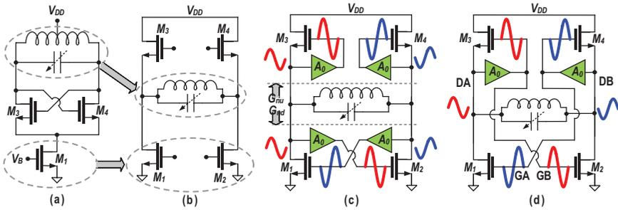
**Figure 6.5** Evolution towards the switching current-source oscillator.
