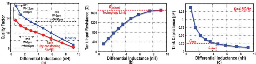
**Figure 6.3** Dependency of various inductor parameters in 28-nm LP CMOS across inductance value: (a) inductor and tank Q-factor; (b) equivalent differential input resistance of the tank; and (c) required tank capacitance at 4.8-GHz resonance. Note that at this point the inductors are without dummy metal fills.
