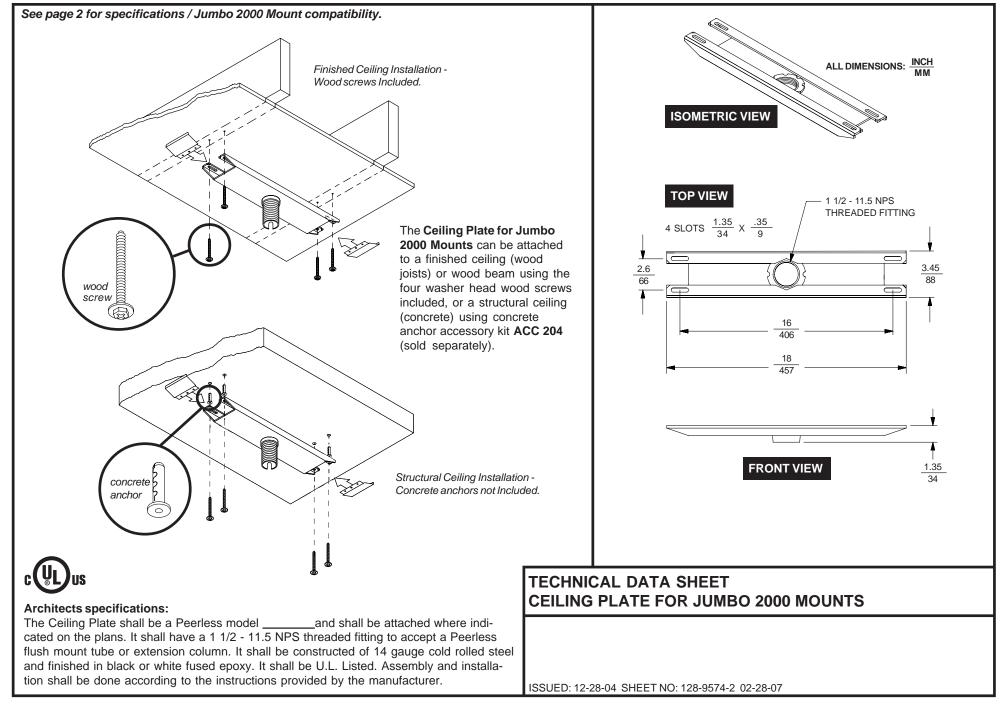
Jumbo 2000 Mount attaches to ceiling plate CMJ 470 or CMJ 470W with flush mount tube or extension column. Flush mount tube is included with Jumbo 2000 Mount. Various
