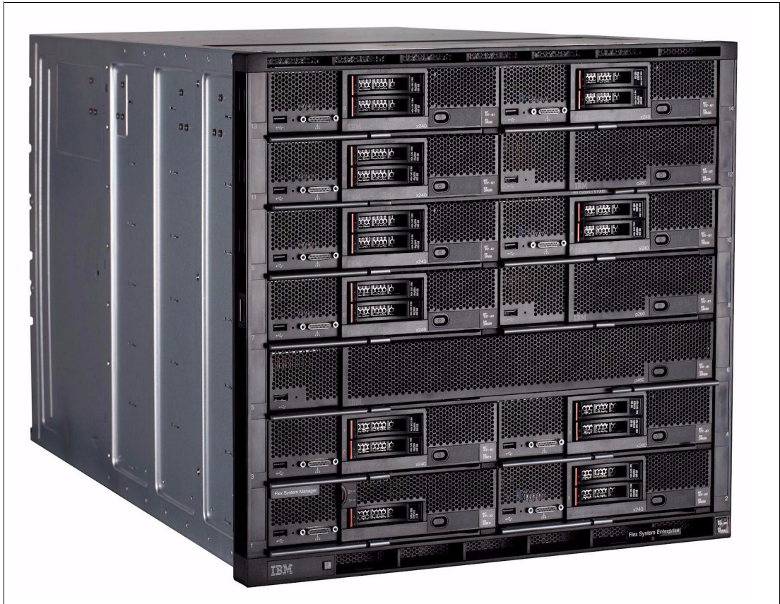
Figure 3-4 IBM Flex System Enterprise Chassis
