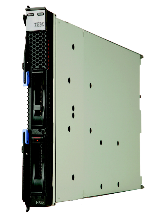
Figure 3-27 Showing the hot swap disk drive bays on the front of the HS12 type 8028
