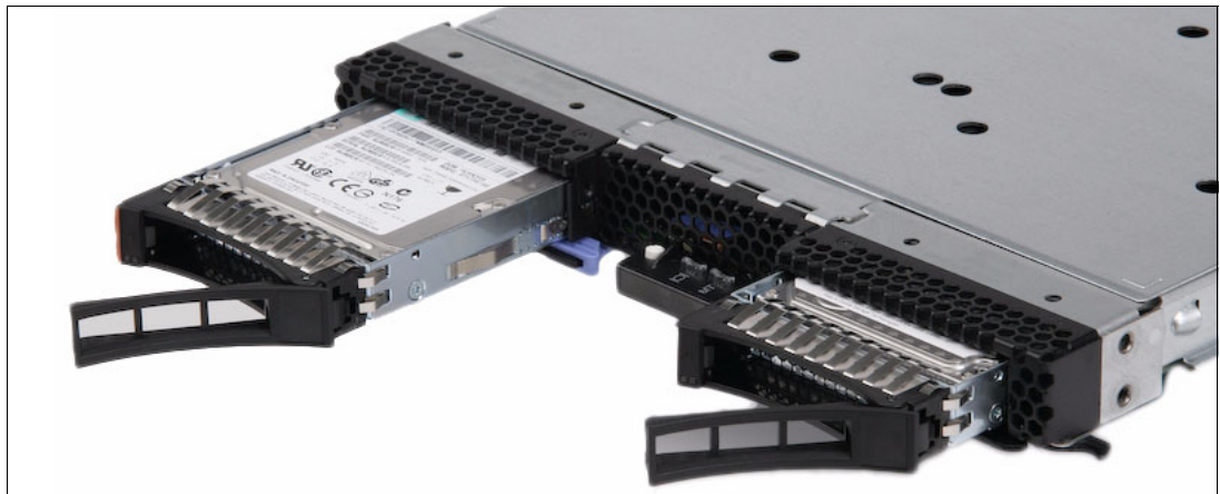
Figure 3-34 The HS22 showing the front hot-swap disk drive bays
