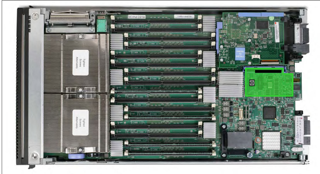
Figure 3-57 The HX5 type 7873 showing the CIOv I/O Expansion card position
