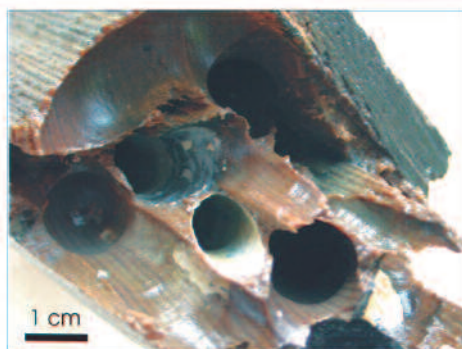
Figure 6. a) Impressions left by soft tube polychaetes in chest components. b) Timber broken as a consequence of teredid activity. One of the tunnels still retains its calcium carbonate lining.
