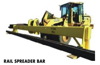
IPS manufactures a wide range of spreader bars for handling rail. A spreader bar that attaches quickly to a forklift is shown. Engineer certified, magnetic particle tested and proof loaded prior to shipping.
