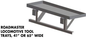
Aluminum locomotive tool tray for engine servicing. Tray measures 41" or 65" wide x 14" deep with 12" high support leg; 2" diameter hook bracket attaches tray to engine safety rails.
