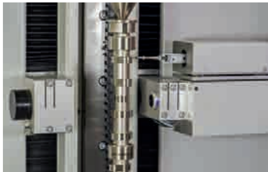
Tactile measuring unit with y-measuring axis 60 mm
