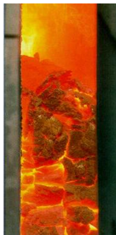
Figure 1: Coke in a Slot Coking Oven
