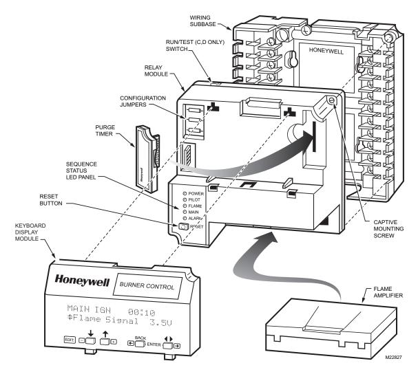
Fig. 4. RM7897A,C Relay Module, exploded view.
