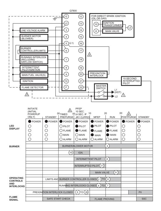
120 VAC, 50/60 HZ POWER SUPPLY. PROVIDE DISCONNECT MEANS AND OVERLOAD PROTECTION AS REQUIRED.
