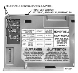
Fig. 15. Selectable site-configurable jumpers.
