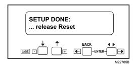
Fig. 13. Release Reset screen.
