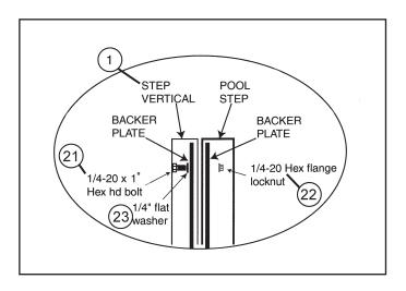
The illustrations show correct hardware placement. CONFIRM BEFORE BEGINNING INSTALLATION
