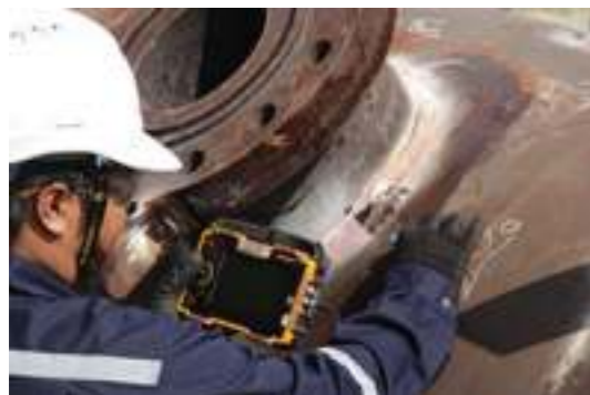
Shear wave are used for flaw detection and longitudinal wave form are used for thickness measurement
