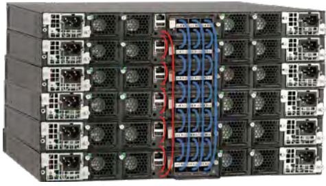
Figure 4: Up to 12 Ruckus ICX 7750 Switches can be stacked using up to 12 standard full-duplex 40 Gbps QSFP+ ports per switch, providing up to 5.76 Tbps of aggregated stacking bandwidth.
