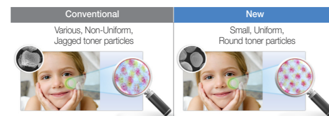
Figure 4. Example of Samsung polymerized toner
