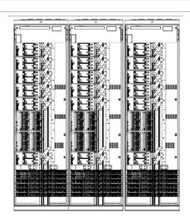
5400A 3 Bay Solution with 72 rectifier slots 75A rectifiers and up to 56 inches of available distribution per bay
