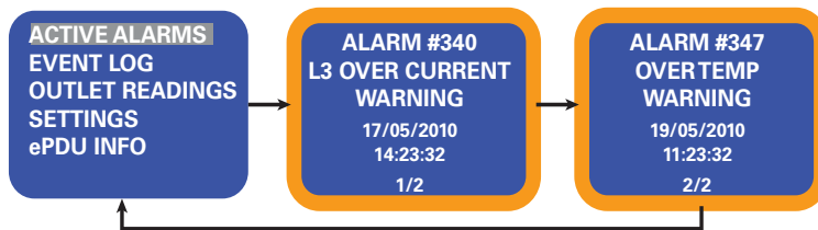
Figure 48. Example Active Alarm Displays
