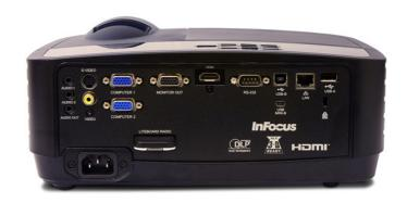
Connectivity VGA x 2 HDMI 1.4 USB-A USB Mini-B Composite Video RJ45/LAN
