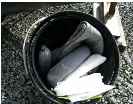
Figure 17: Typical Spill Kit contents
