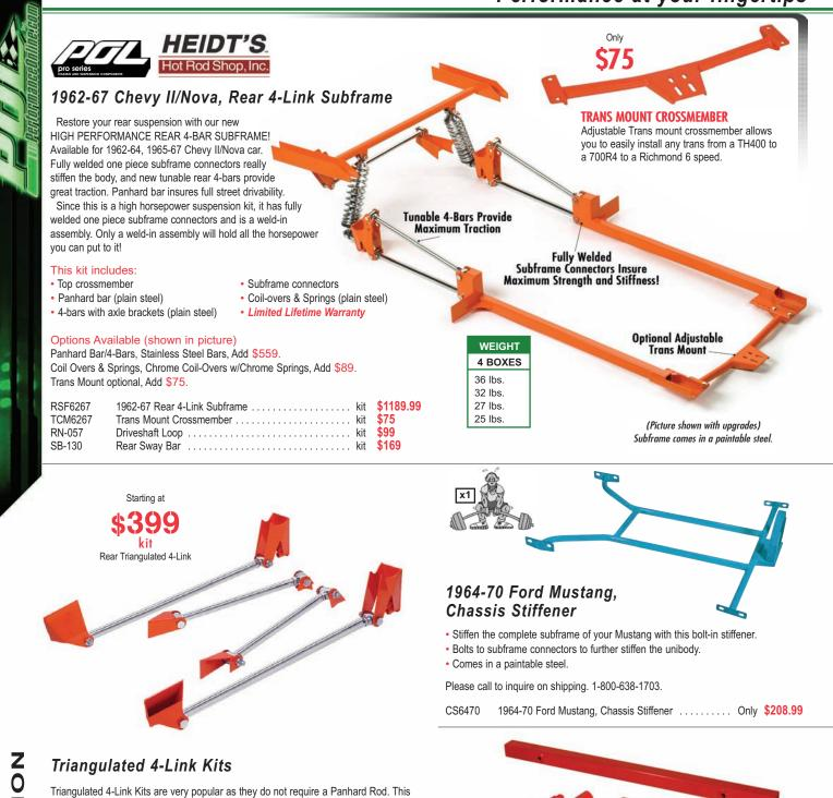
Triangulated 4-Link Kits are very popular as they do not require a Panhard Rod. This design is also similar to many GM installations. Bars are fully adjustable, 1" X .156 tube with 3/4" stainless adjusters and urethane bushings, angled and straight chassis brackets, multi-position coil-over axle brackets, tabs and hardware. These kits are available in plain steel or polished stainless steel tubes. Intended for fully boxed or aftermarket frames.
