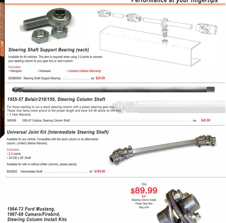
This item is required when adding power steering to your Camaro/Firebird or Ford Mustang car. Please specify tilt or tilt w/shift column. Does not require a wire harness adapter. (Please specify steering box, steering column being used and year of vehicle. To be used in conjunction with tilt column).
