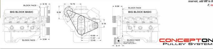
Just like the small block basic kit, this basic serpentine pulley kit is a two-belt kit designed for those who want a neat, compact alternator only or alternator and power steering setup without air conditioning. The alternator fits tightly in front of the passenger side head. The power steering pump, if equipped, mounts low on the block on the drivers side. For kits not equipped with power steering, a single belt is placed on the back groove of the crank and waterpump pulleys.
