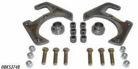
Uses: 73-91 F-100 rotors, 71-87 GM C-10 calipers
