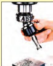
4. Inserting endmill holder & endmill for next operation
