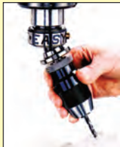
2. Loading drill chuck holder & drill into body
