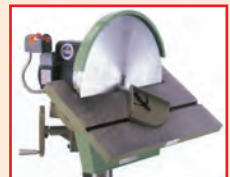
Tilts downward a full 45° Tilts upward 35°
