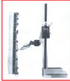
Calibration of Height Gage using vertical position
