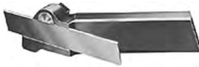
Offset: Straight, Right hand (Shown) or Left hand cutting.
