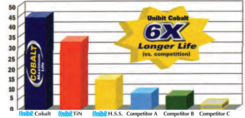
Average Number of Holes Before Failure (In 16 Gauge Stainless Steel Plate)
