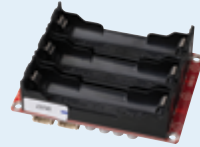
Dayton Audio KAB-BE 18650 Battery Extension Board for KAB Amplifier Boards
