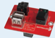
Dayton Audio KAB-INT Interface Extension Board for Bluetooth Amplifier Boards
