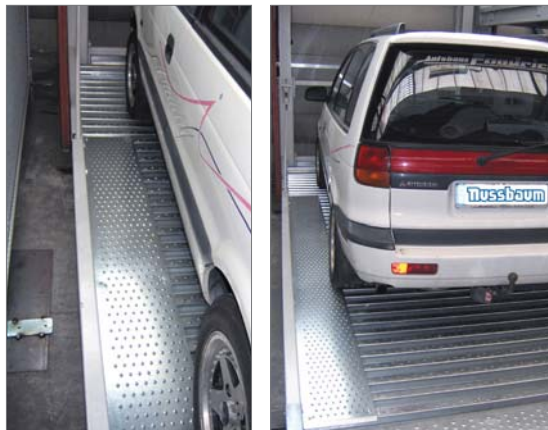
Positioning on the left side of the parking space even more comfortable, when walking to the driver's door. 1,5mm zined sheet, surface are coined. The catwalks are screwed to the driving plates, available with corrosion protection version "Classic" or "Classic Plus". Dimensions: approx. 350cm x 31/41 cm (L x W)
