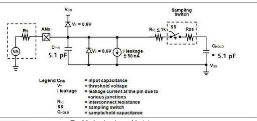
Fig.39: Analog Input Model
