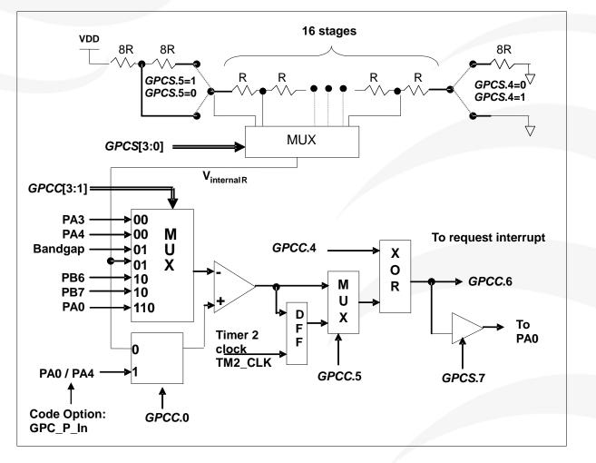
Fig. 29: Hardware diagram of comparator
