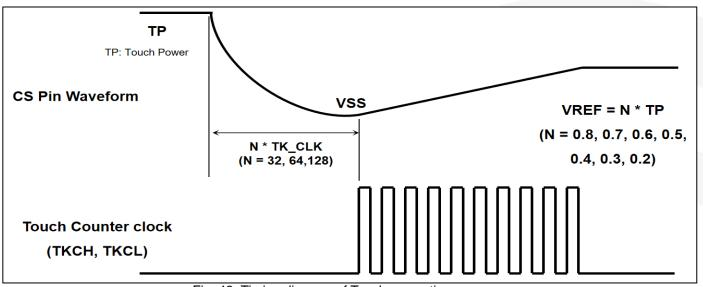
Fig. 42: Timing diagram of Touch converting progress
