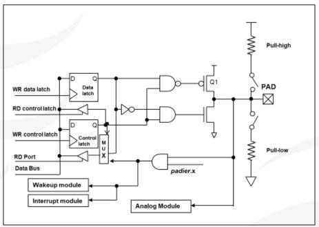
Fig. 16: Hardware diagram of IO buffer
