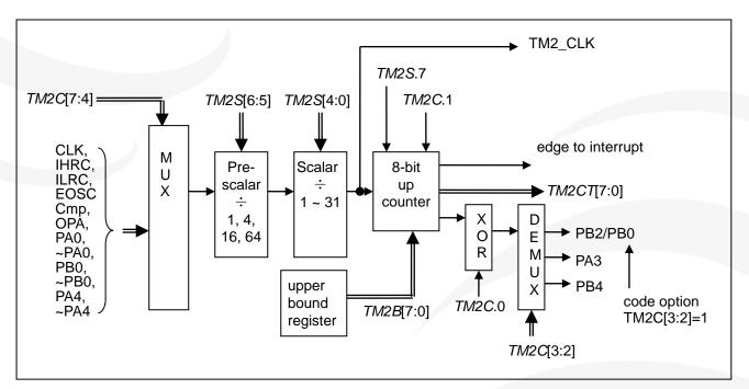
Fig. 18: Timer2 hardware diagram
