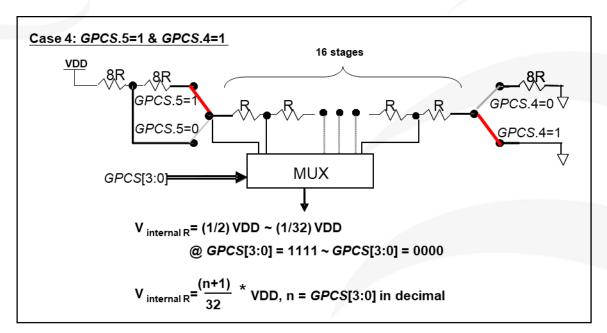
Fig. 34: Vinternal R hardware connection if GPCS.5=1 and GPCS.4=1
