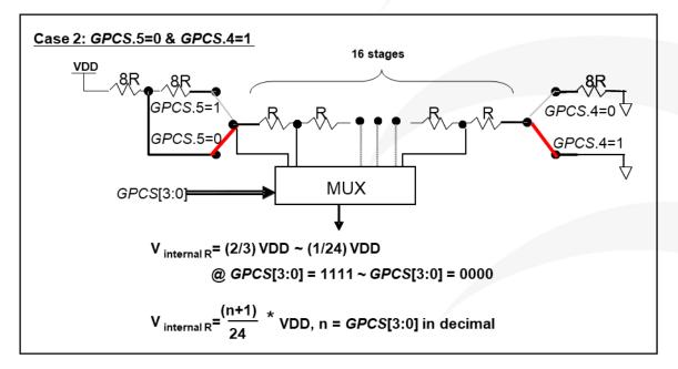
Fig. 32: Vinternal R hardware connection if GPCS.5=0 and GPCS.4=1
