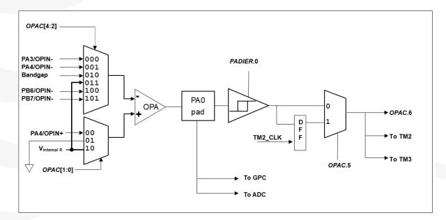
Fig. 36: hardware diagram of OPA
