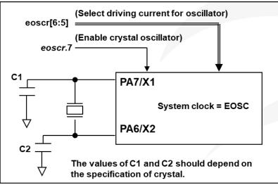
Fig. 8: Connection of crystal oscillator
