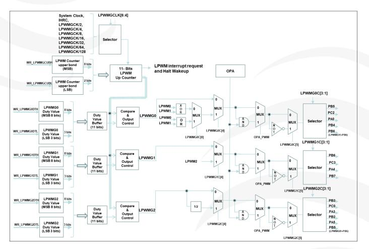
Fig. 25: Hardware Diagram of three 11-bit LPWM Generators
