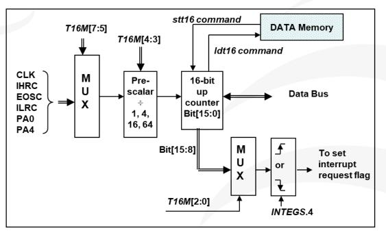
Fig. 17: Hardware diagram of Timer16
