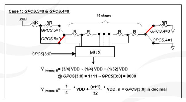
Fig. 31: Vinternal R hardware connection if GPCS.5=0 and GPCS.4=0
