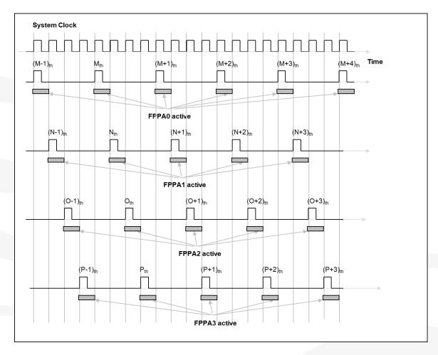
Fig. 2: Hardware and Timing Diagram of four FPPA units
