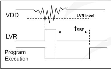
Fig. 12: Low Voltage Reset Sequence
