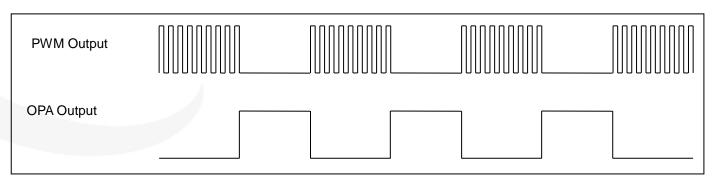
Fig. 37: OPA comparator mode control PWM output
