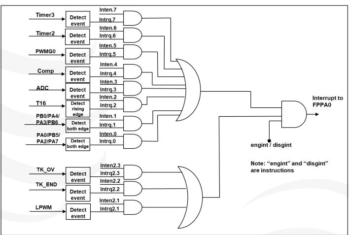
Fig. 15: Hardware diagram of Interrupt controller
