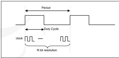
Fig. 20: PWM Output Waveform
