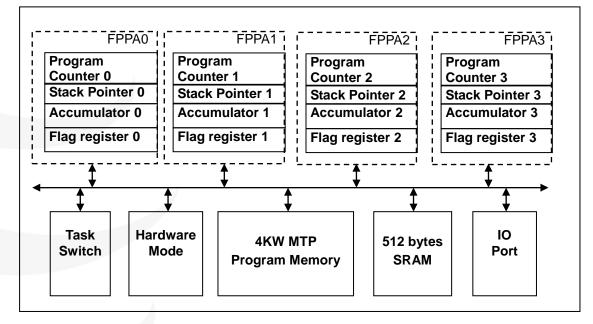
Fig. 1: Hardware Diagram of FPPA units
