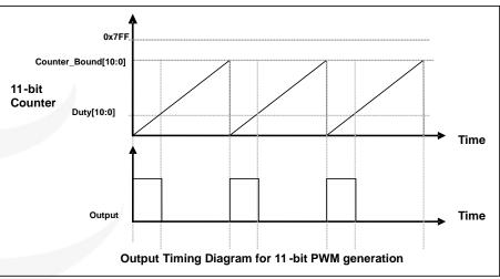
Fig. 22: Output Timing Diagram of 11-bit PWM Generator
