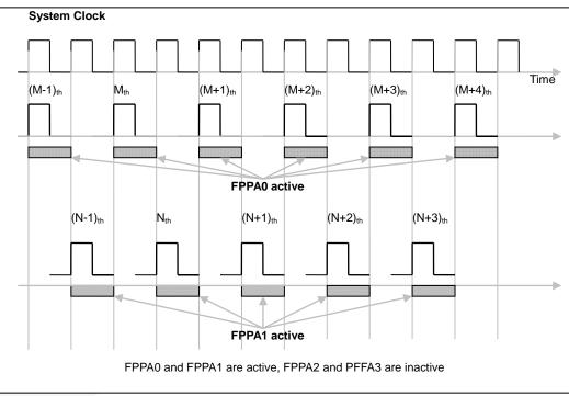
Fig. 3: Hardware and Timing Diagram of two FPPA units
