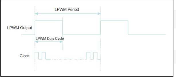
Fig. 24: PWM Output Waveform
