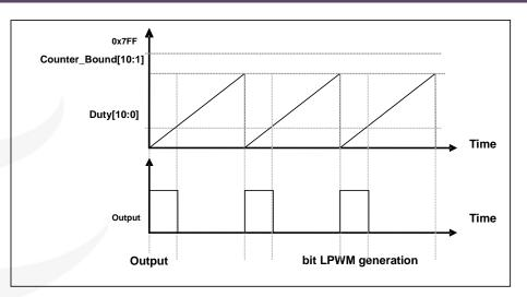
Fig. 26: Output Timing Diagram of 11-bit LPWM Generator
