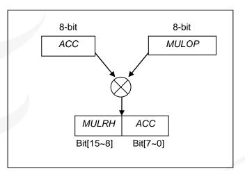
Fig. 40: Block diagram of hardware multiplier
