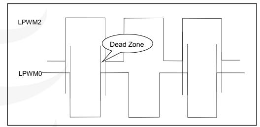
Fig.27: Complementary LPWM waveform with dead zones
