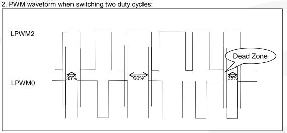
Fig.28: Complementary LPWM waveform with dead zones
