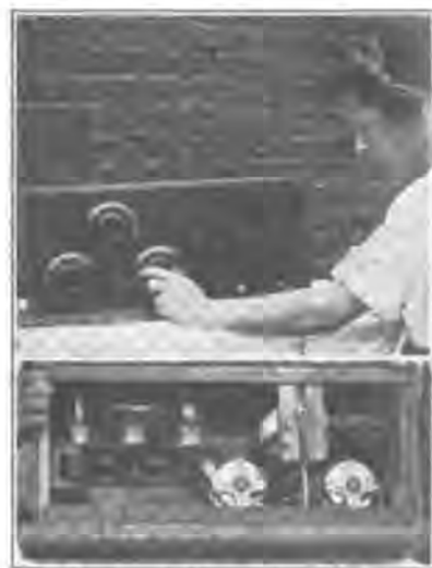
Front and Rear View of Set as the vernier. The variometer controls the regeneration.
