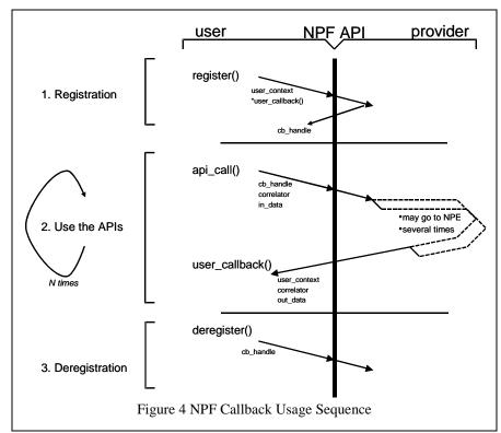
There need not be a 1:1 relationship between an asynchronous request call and a completion callback. A single request call may generate multiple asynchronous response callbacks. Partial completions may happen, for example, when there are multiple input arguments in the request, and the implementation
