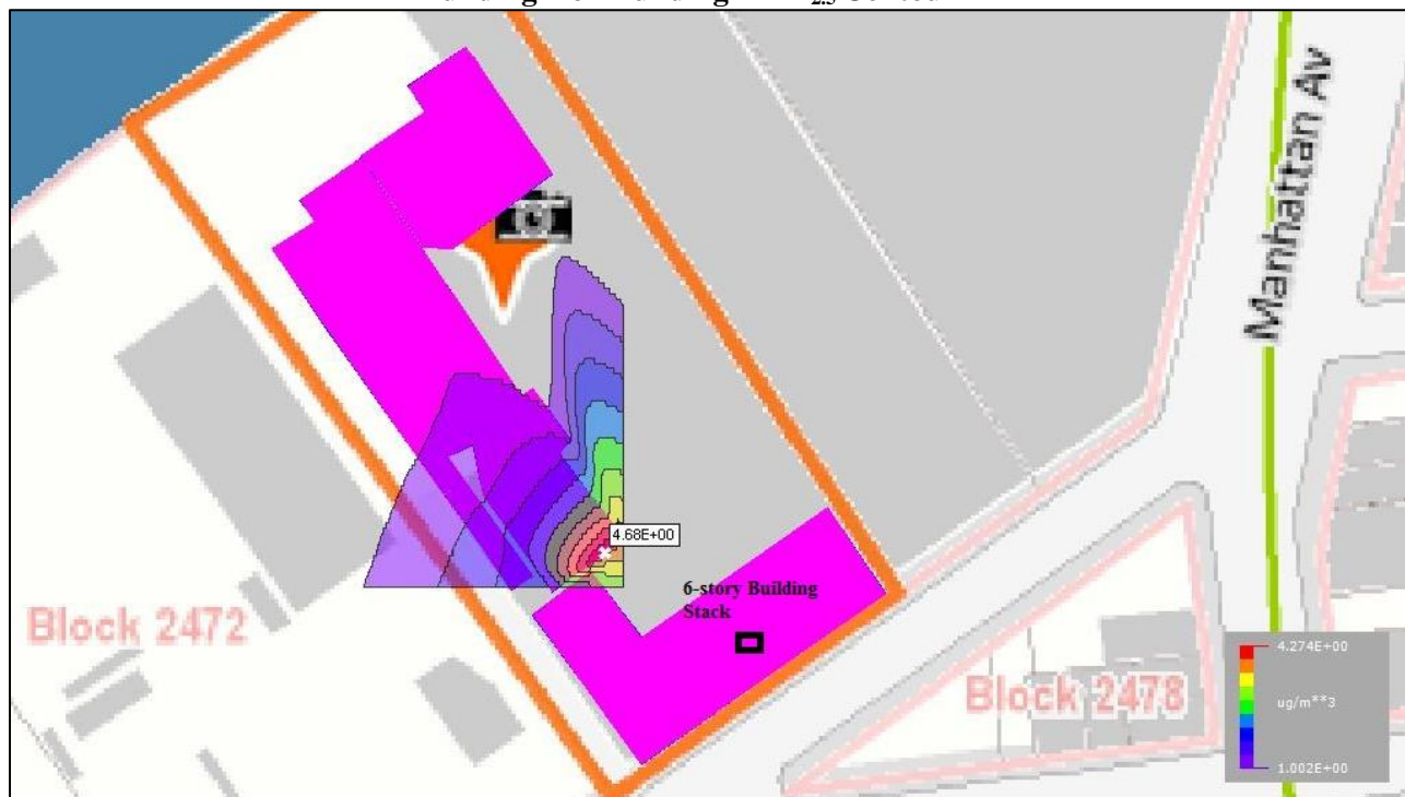
Figure I-5 Building 1 on Building 2 PM 2.5 Contour
