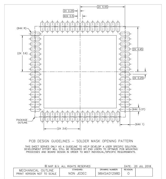
Figure 49. Reflow soldering footprint part 1 for HVQFN64 (SOT804-3(D))
