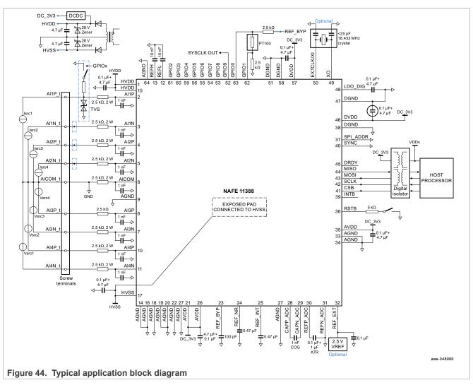
Note: Dash boxes on AI1N, AI2P, AI2N inputs represent the dashed circuitry on AI1P.
