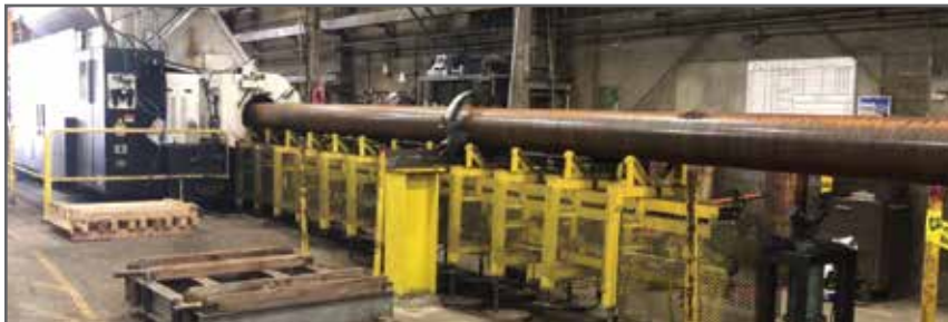
Nucor Skyline can provide threaded micropile casing up to 40 feet.
