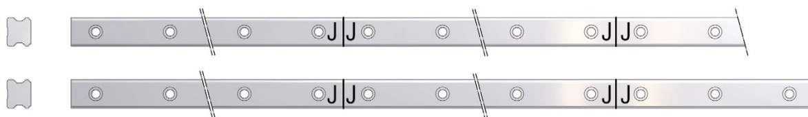
Figure 3.6 Marking of jointed rails
