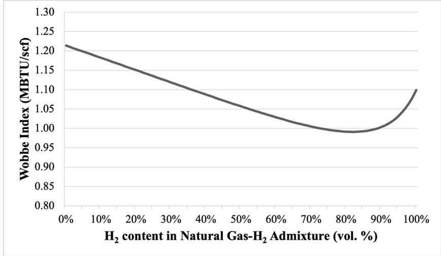
Figure 3. Effect of hydrogen composition on Wobbe Index.
