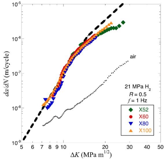
Figure 5. Fatigue crack growth of a diverse range of pipeline steels in gaseous hydrogen (San Marchi and Ronevich 2022).
