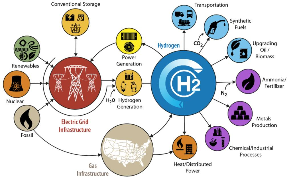
Figure 1. Hydrogen production and utilization pathways (Ruth et al. 2020)
