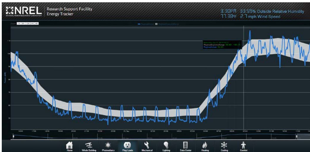
Figure 4–8 Plug loads predicted range visualization with measured use (blue line) and control limits (silver band) for September 24, 2013 14:00 to September 25, 2013 14:00
