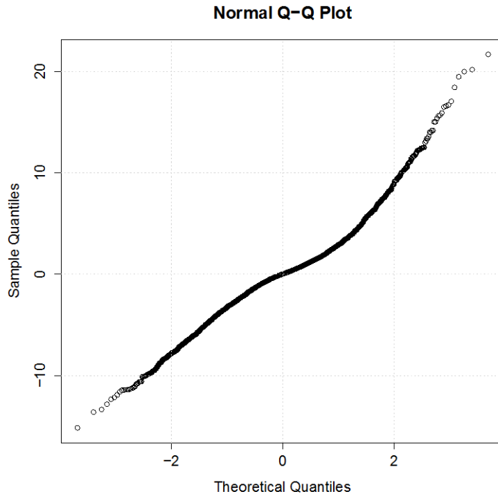
Figure 6–5 Q-Q normal plot for residuals of linear model for measured cooling energy end use during occupied periods
