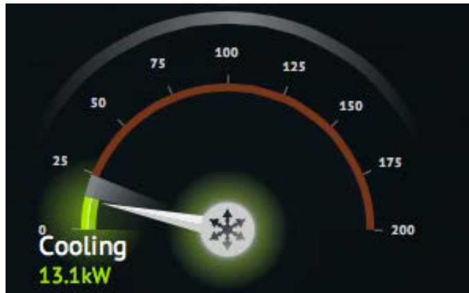
Figure 5–26 Dashboard view of instantaneous total cooling power (kW) in the RSF along with LCLs and UCLs shown as a gray band above
