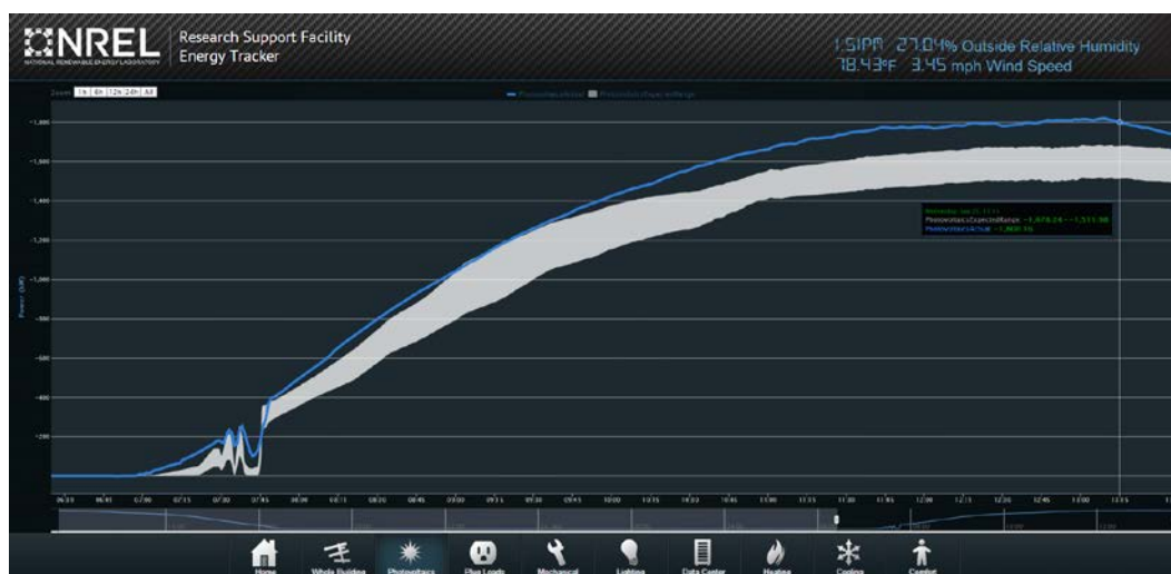
Figure 4–2 PV production predicted range visualization, blue line (measured) and silver band (control limits) for September 25, 2013
