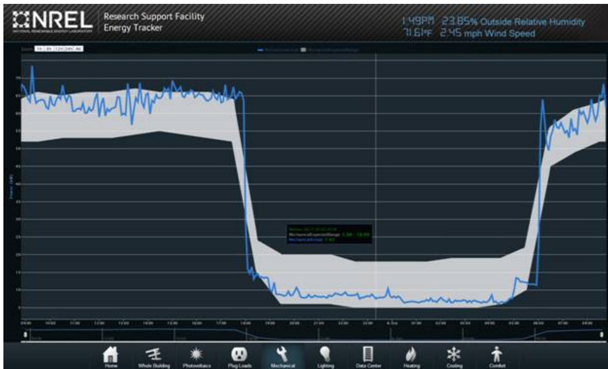
Figure 4–11 Mechanical systems predicted range visualization with measured use (blue line) including corrected air handler schedule and control limits (silver band) on October 7 and 8, 2013
