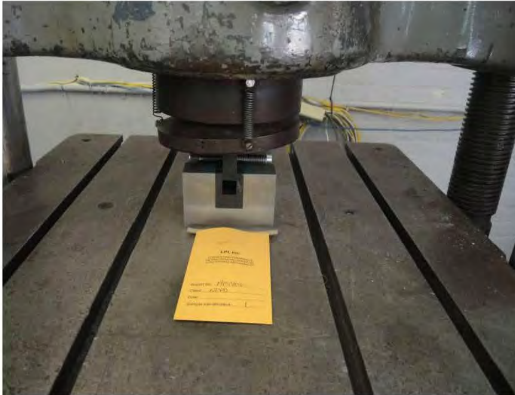
Figure C-2: Testing of Bolt #1 (as an example)
