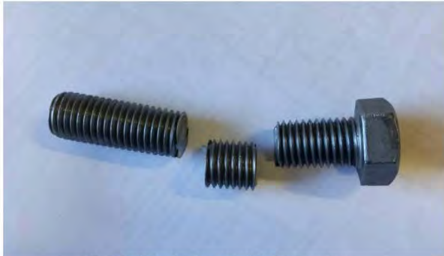
Figure C-3: Broken Bolt After Testing (Bolt # 1 as an example)
