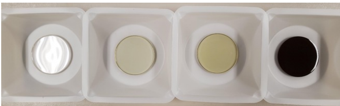
Figure 7. Photograph of 40 mm diameter, homogeneous lithium borate flux beads made from (Bottom: Left to Right) flux blank with no sample added, TCG, TCG-NBFS, and an iron steel slag material.
