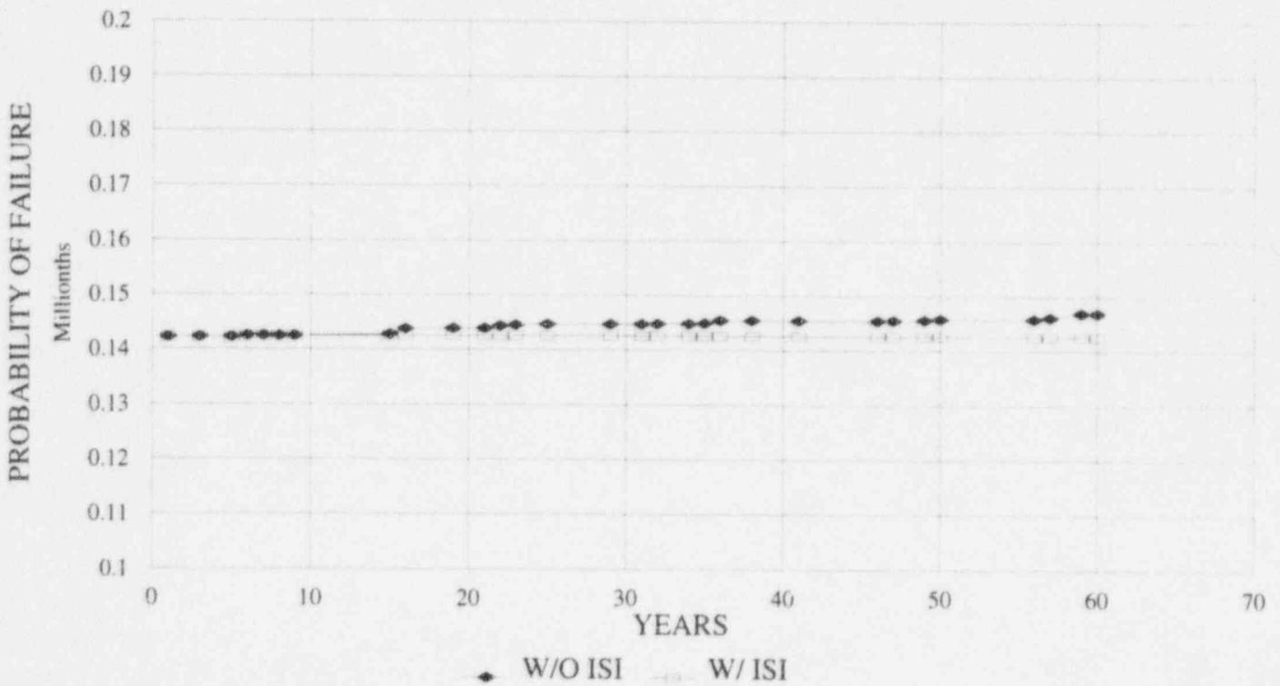
Figure 5-7: Probability of Failure for Flywheel Evaluation Group 2
