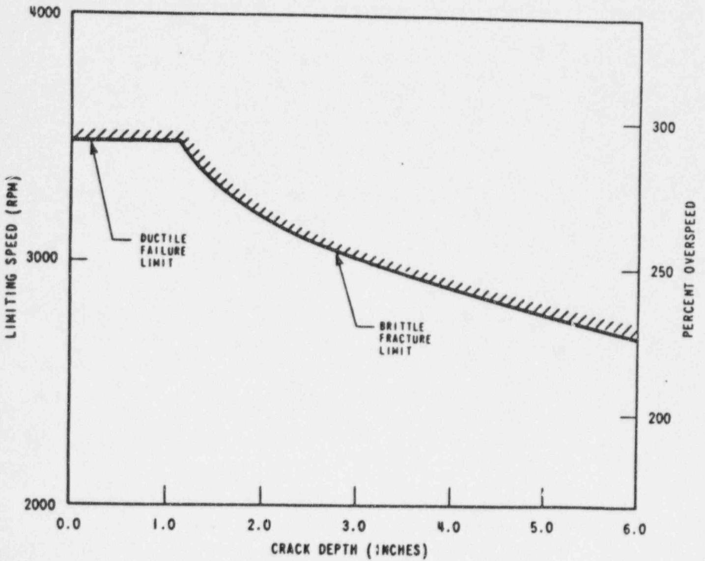
Figure 4-1: Results of a Typical Reactor Coolant Pump Flywheel Overspeed Evaluation
