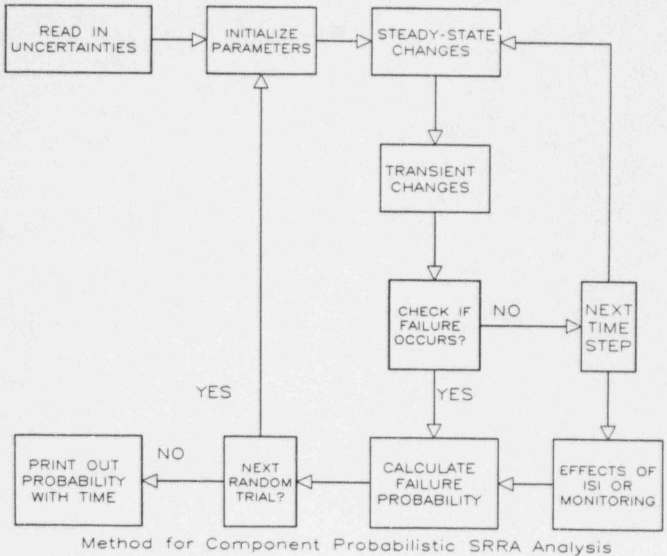
**Figure 5-4: Westinghouse PROF Program Flow Chart for Calculating Failure Probability**
