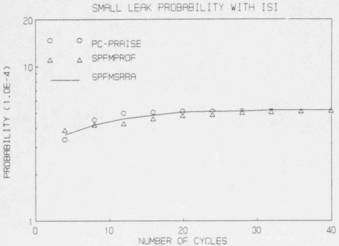
**Figure 5-3: Comparison of Leak Probabilities with Inservice Inspection**
