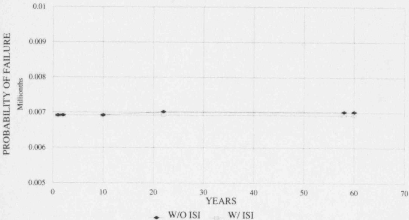
Figure 5-11: Probability of Failure for Flywheel Evaluation Group 16
