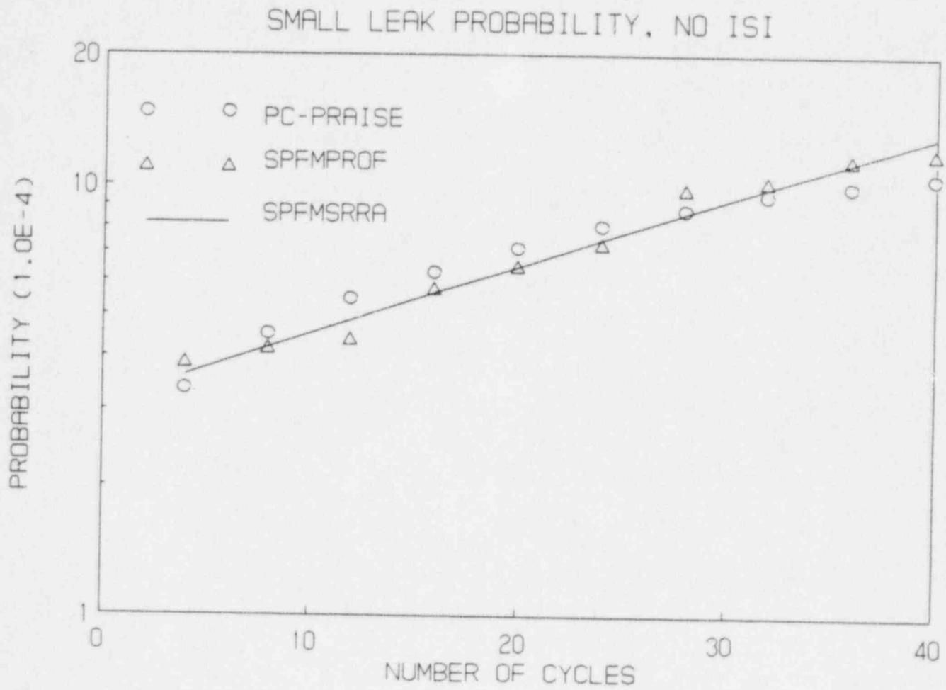
Figure 5-2: Comparison of Leak Probabilities without Inspection
