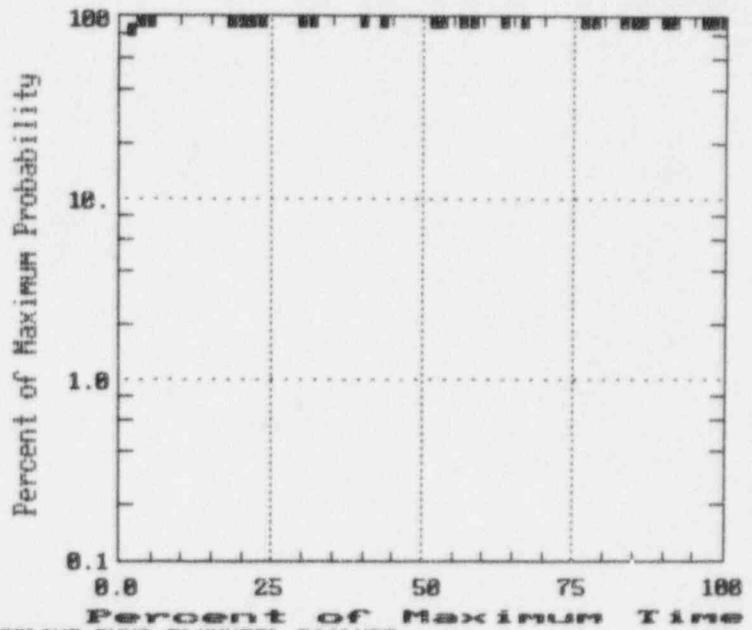
Figure 5-5: Computer SRRA Plot for RCP Flywheel Failure Probability
