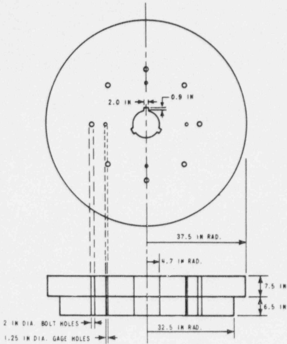
Figure 2-1: Example of a Flywheel which is Attached Directly to the Motor Shaft
