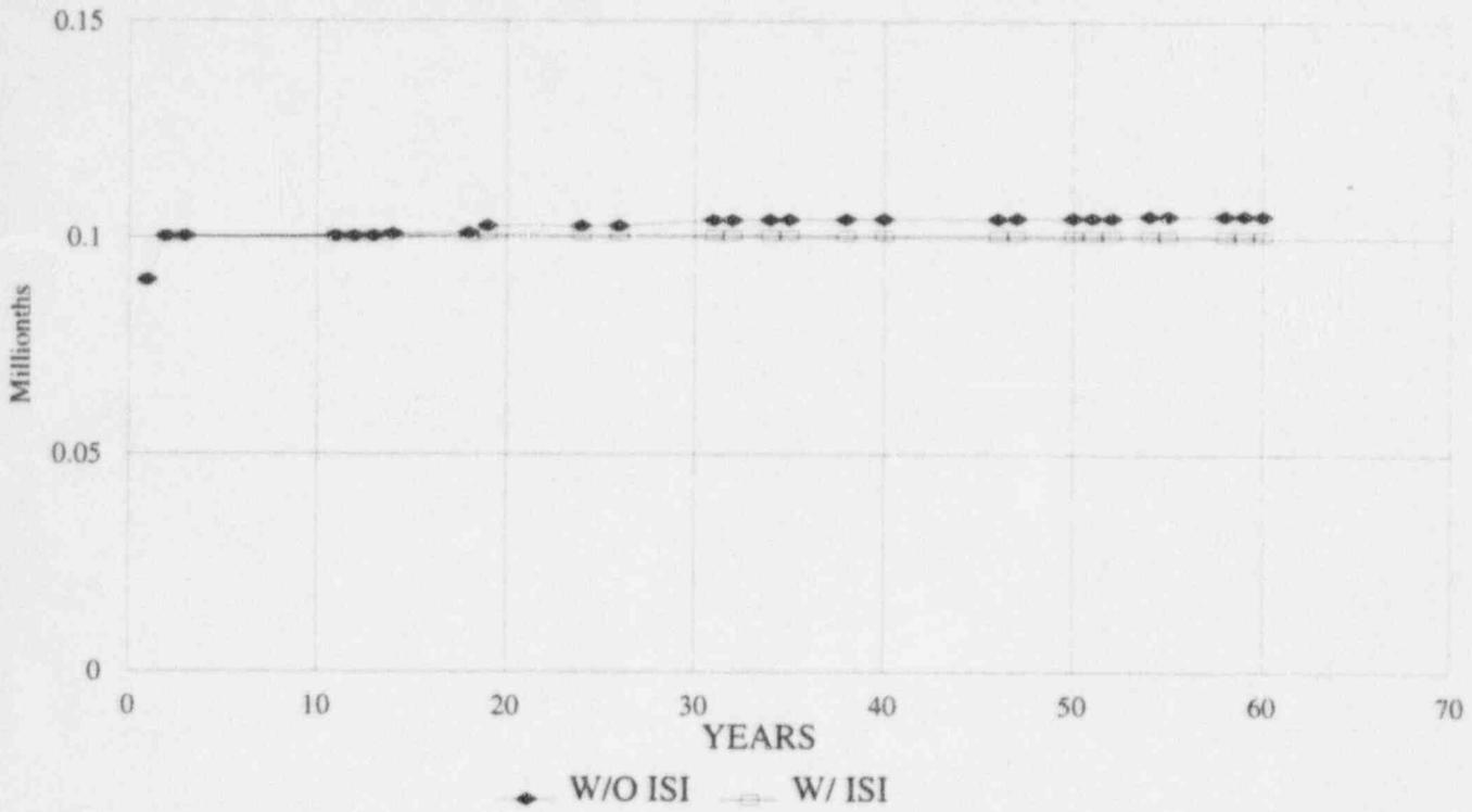
Figure 5-8: Probability of Failure for Flywheel Evaluation Group 10
