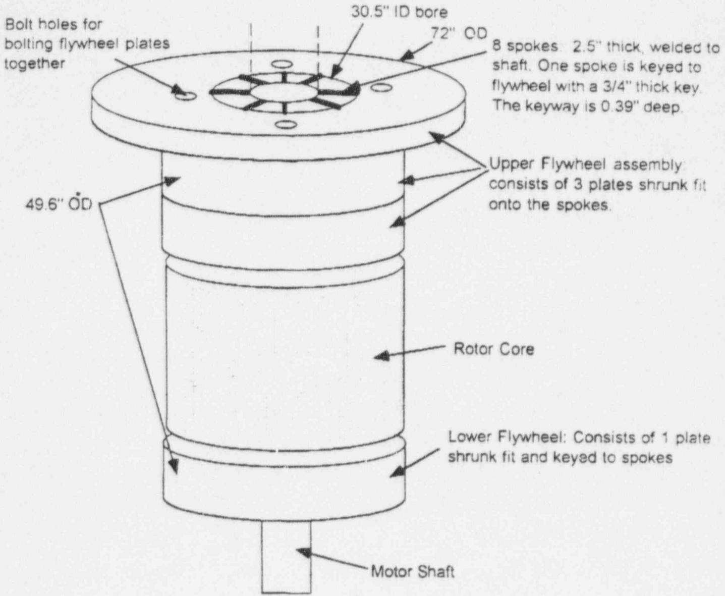
Figure 2-2: Example of a Spoked Flywheel
