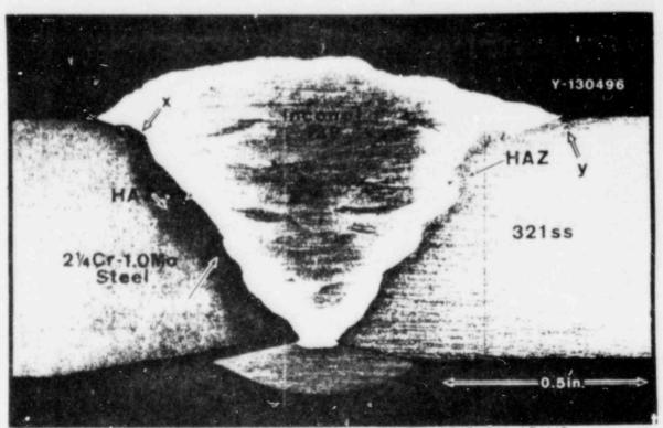
LONGITUDINAL CROSS SECTION OF TRANSITION JOINT Areas designated "x" and "y" receive specific attention in this examination, Heat Affected Zones (HAZ) in the 2 1/4 Cr-1.0 Mo steel and type 321 stainless steel are indicated.
