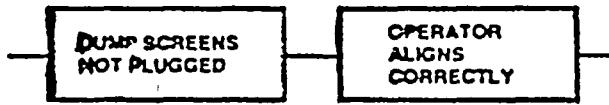
Figure A1.2.8 Logic diagram for top event RF Operator aligns system for recirculation and sump screens remain unplugged
