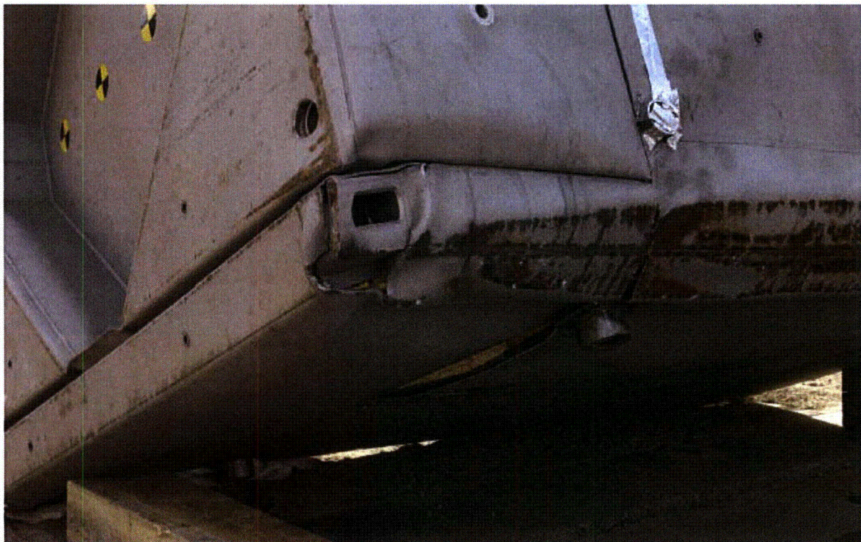
Figure 3.5-20 – Weld Tear from LD-5 Free Drop Orientation
