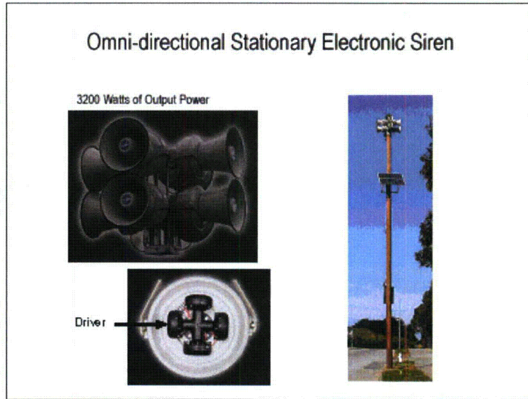
Figure 8-1. Typical Stationary Omni-Directional Siren in New System
