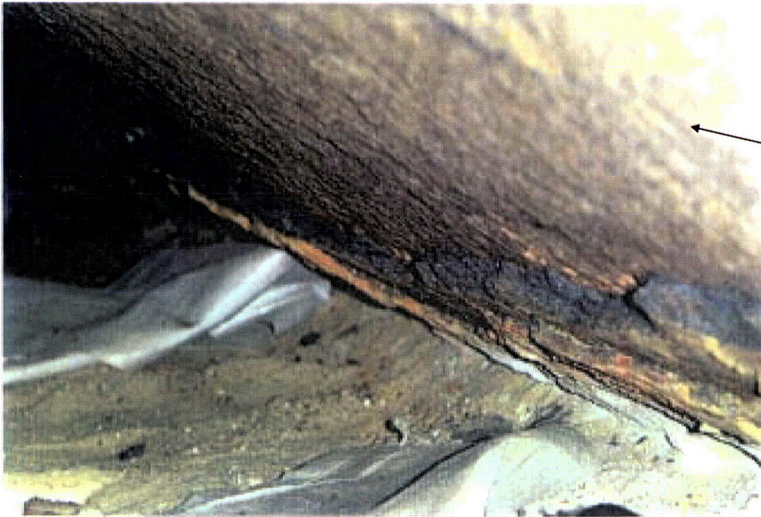
Corrosion product on drywell vessel
