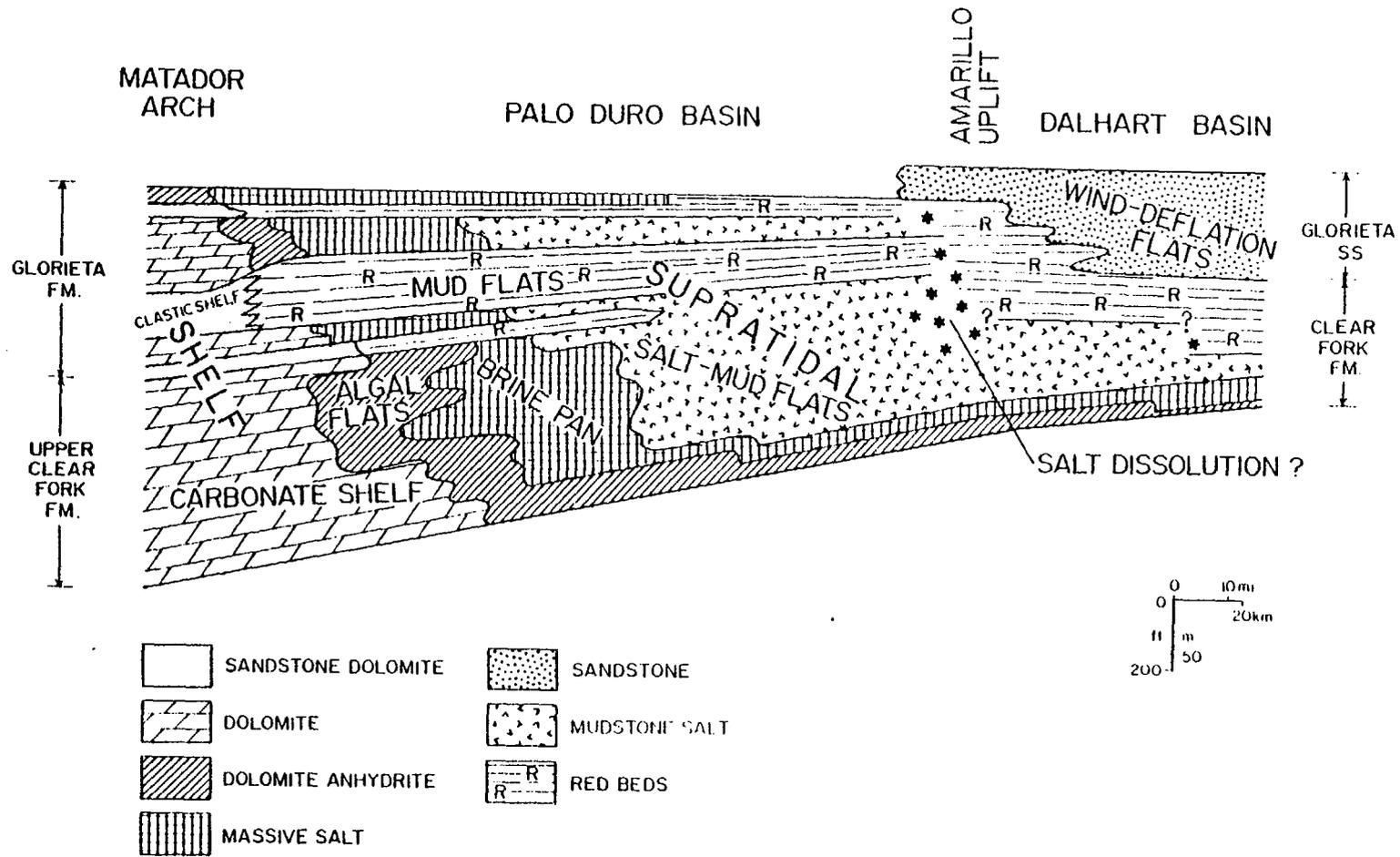
Figure 43. North-south facies cross section through Palo Duro and Dalhart Basins showing relation of environments for the upper Clear Fork and Glorieta Formations. From Presley (unpublished data).
