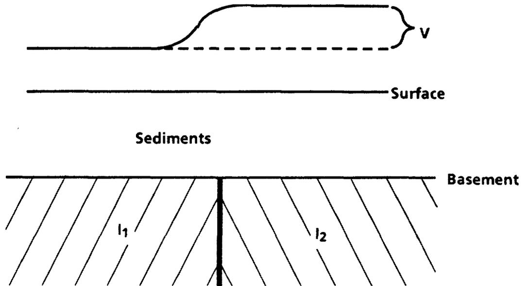
$$\begin{aligned} V &= 2\pi (I_1 - I_2) && \text{(Nettleton, 1976)} \\ &= 2\pi (0.002) && \text{(Nettleton, 1976)} \\ &= 0.1256 \text{ gauss} = 1256 \text{ gammas} \end{aligned}$$
