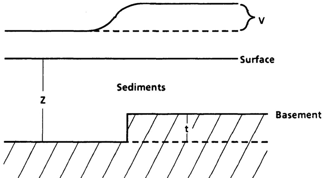
$$\begin{aligned} V &= 2It/Z && \text{(Nettleton, 1976)} \\ &= 2(0.002)(1000)/8000 \times 10^5 \\ &= 50 \text{ gammas} && \text{for } t = 1000 \text{ feet} \\ &= 100 \text{ gammas} && \text{for } t = 2000 \text{ feet} \end{aligned}$$
