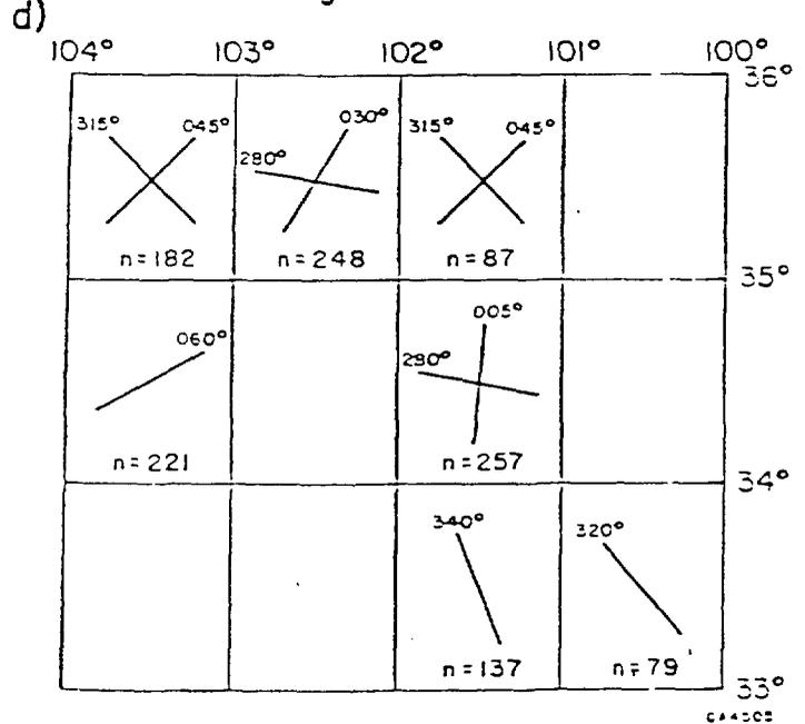
Figure 3 Fracture maps of the Texas Panhandle and eastern New Mexico region showing (a) mean fracture strikes for Permian strata, (b) mean fracture strikes that are significant at 95% confidence for Permian strata, (c) mean fracture strikes for Triassic strata and (d) mean fracture strikes that are significant at 95% confidence. Stations for fracture measurements and structural setting are shown in figure 1. n = the number of measurements in each quadrant.
