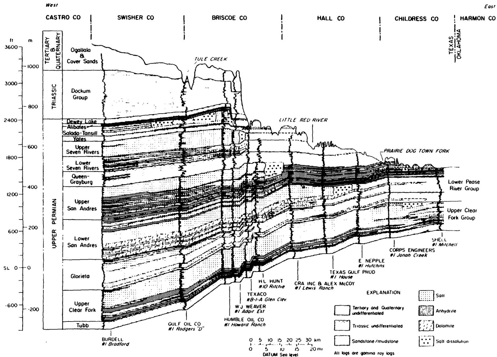
Figure 2. Structure and stratigraphic cross-section on the northeast flank of the Palo Duro Basin.
