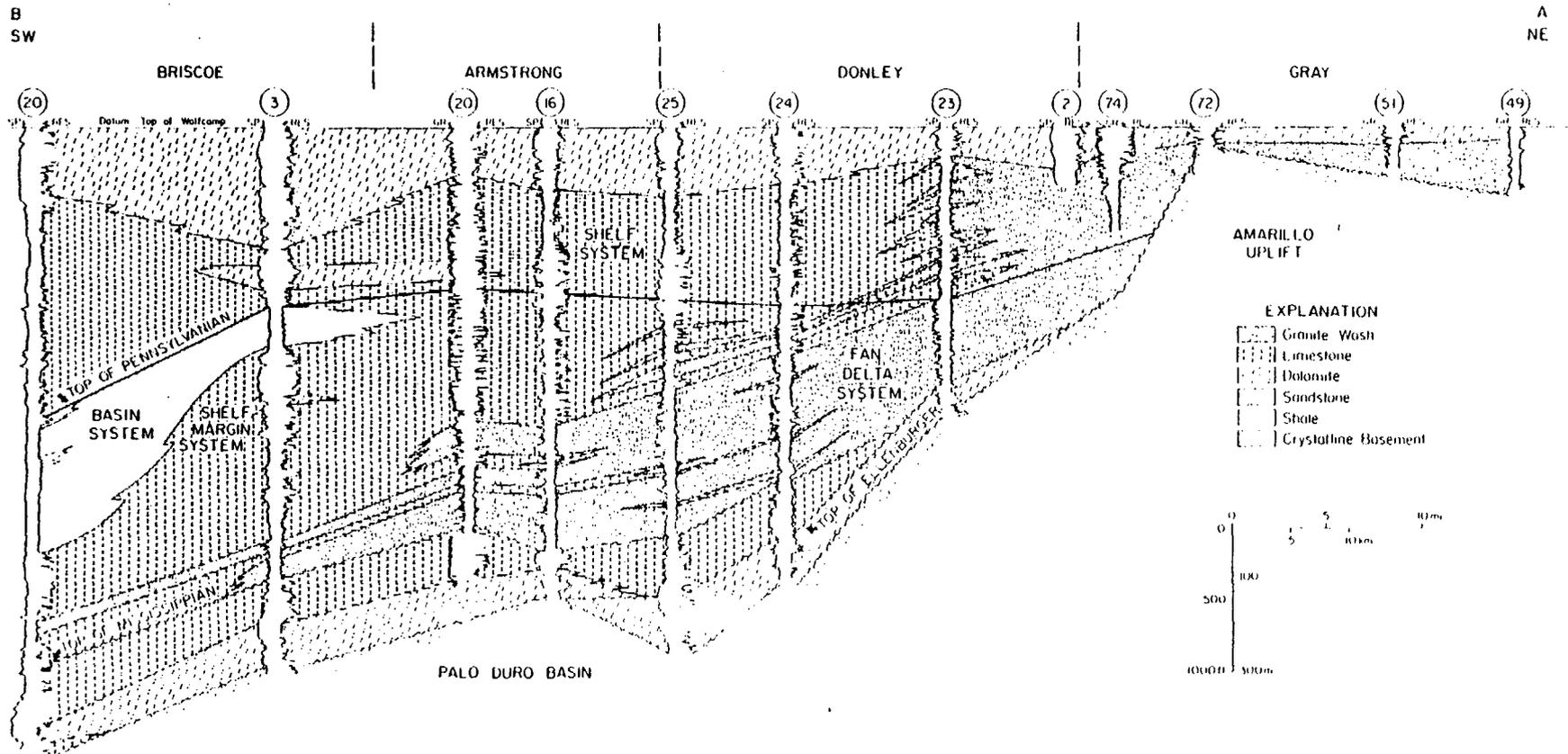
Figure 59. North-south regional cross section A-B from the central Palo Duro Basin to the Amarillo Uplift. Line of section shown in figure 57.
