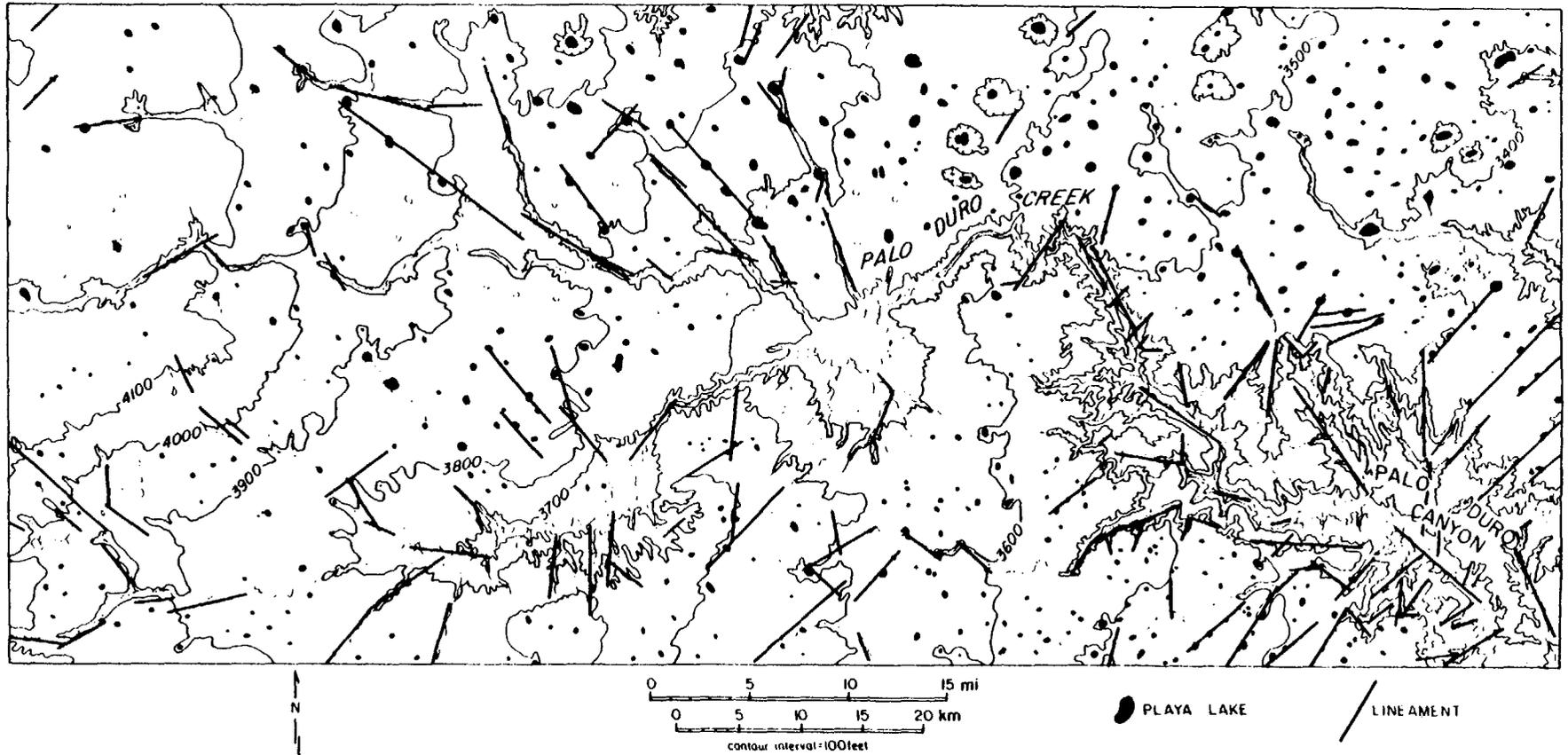
Figure 3. Detail of lineaments mapped on Landsat imagery in the vicinity of Palo Duro Creek and Palo Duro Canyon. Linear stream segments and escarpments form many of the lineaments. Area shown is A in figure 4. Original imagery is at a scale of 1:250,000.
