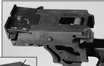
An unusual feature of the IZH-35M target pistol is the hammer, which is hinged at the top to swing downward to strike the firing pin. That allows the top surface of the hammer (arrow) to serve as a cocking indicator.
