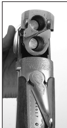
Fausti/Traditions over-under shotguns are conventional box locks with Kersten locking and top lever operation. The hook-shaped Kersten locks recline into vertical slots cut into the breech face where cross bolts assure a tight lockup.
