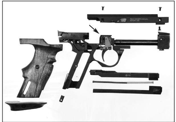
Designed from the ground up as a target pistol, the IZH-35M is blowback operated with a fixed barrel silver soldered into a barrel mounting block (arrow) which is an integral part of the frame. The front sight is mounted on a second block pinned to the muzzle.
