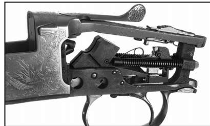
Fausti/Traditions over-under shotguns are conventional box locks with Kersten locking and top lever operation. The hook-shaped Kersten locks recline into vertical slots cut into the breech face where cross bolts assure a tight lockup.
