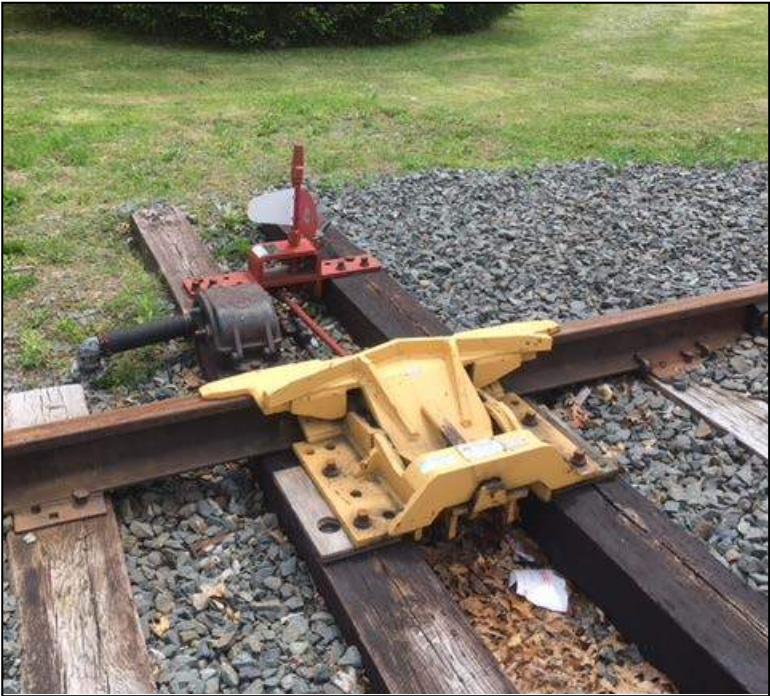
6b. Sliding Block Derail
