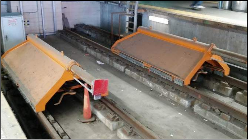
8b. High Energy Hydraulic Bumping Post
