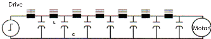
Figure 5: Delay Line Equivalent Circuit of Long Cable
