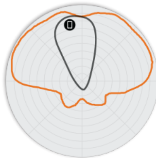
Figure 4. R710 2.4GHz Elevation Antenna Patterns
