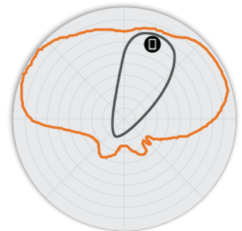
Figure 5. R710 5GHz Elevation Antenna Patterns
