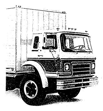
Figure 2-3. Truck With Low Deck Cab-Over-Engine
